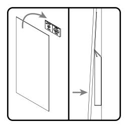
6. Peel the protective cover strip from the double sided tape on the support brackets.
