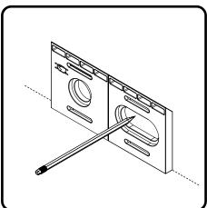
3. Drill holes to a depth of 1  $^{3}$ / $_{4}$ " (45mm) and insert the wall plugs level with the surface of the wall. (Note: if you are fitting the product to a tiled surface, insert the wall plugs below the surface of the tile to avoid cracking the tiles). Insert the countersink screws through the Hang 'N' Lock cams and loosely secure the Hang 'N' Lock bracket to the wall.
