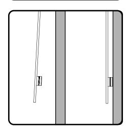
8. The wall spacer can be screwed to the wall if the mounting surface is unsuitable for fixing with adhesive tape.
